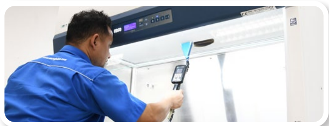
Figure 5. Filter integrity test conducted by a trained and certified engineer.
