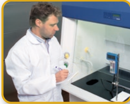
Face velocity measurement test
