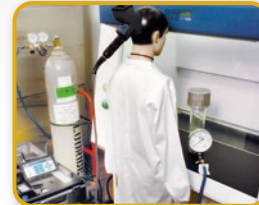
Tracer gas containment test
