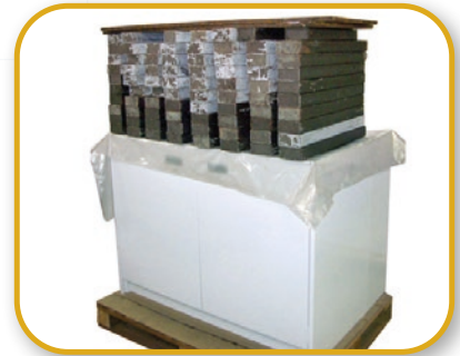
Cabinet Load Test
